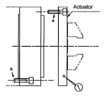
Attach the actuator and then check that it is centered to a deflection of no larger than about 5 microns. For higher accuracy or finishing the jaws, use the bolt "a" to center the actuator. Check actuator the centered to a deflection of no larger than 1 micron. If the actuator is not centered to that level, use the bolt "b" to perform centering.
