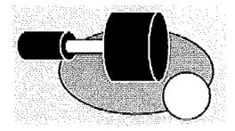
The parts for VIDA CLAMP may be damaged during machining, causing the workpiece and those parts to be scattered around.
